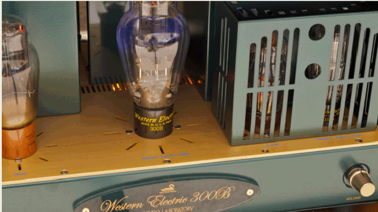
The legendary Shindo Western Electric 300B Limited Mono Block Amplifier. Ken Shindo designed his first 300B single ended amplifier in 1979. Continually refined over the years, the WE 300B Single Limited is the flagship Shindo amplifier. Genuine NOS Western Electric 300B tubes from the original production run are employed for 8 watts Class A output. Speakers of 90db sensitivity or higher are recommended.
